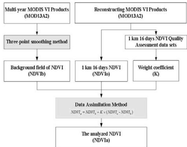
Fig.1. The flowchart of reconstructing MODIS NDVI data
