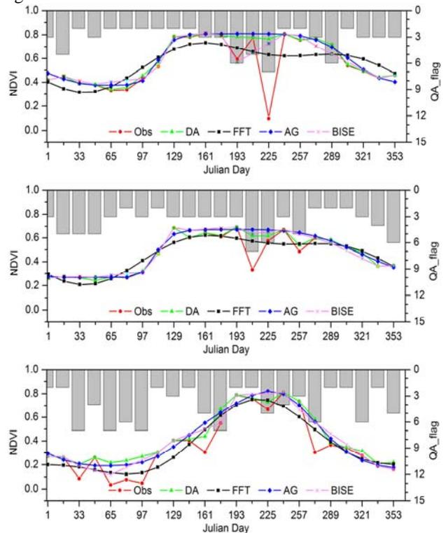
**Fig.3. The final NDVI time series of three test points generated by the new method, the FFT method, the asymmetric gauss fitting and the BISE algorithm.**
