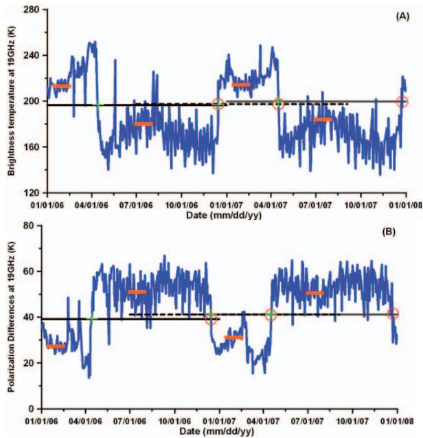
Figure 1 Examples of the dynamic thresholded algorithm to monitor the freeze-up and break-up dates of lake ice over the Lake Balkhash. (A) Brightness temperature (Tbs) and (B) polarization differences (PDs).
