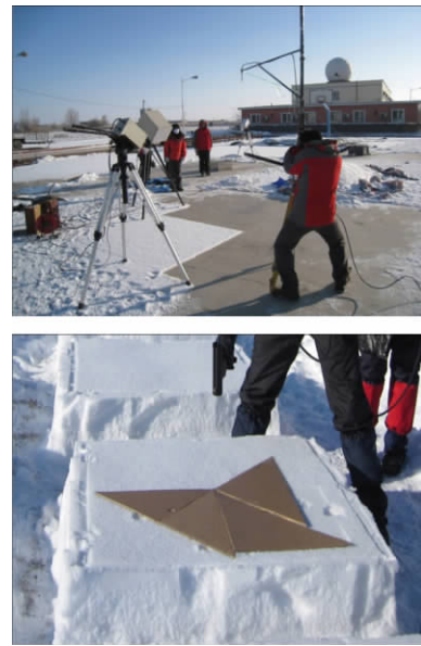
Fig 2 The in situ measurement of spectral reflectance of different fractional snow cover
